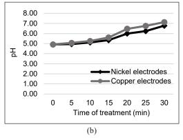
Figure 2. Graph of the effect of electrocoagulation treatment using nickel and copper electrodes on (a) Turbidity; and (b) pH of pepper wastewater
